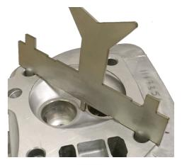
The spark plug insert must show a clearance to the CPO gauge, which must be flush on the cylinder face
