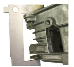
When placing the CPO gauge over the rocker cover face, the lower lip must not engage over the cylinder mating face
