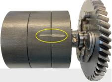
segments of the gauge to their respective camshaft lobes. All segments of the gauge must be an easy fit, and no rocking or other manipulation can be utilised to enable the gauge to fit.
