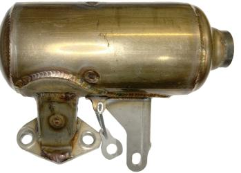
in place at all times. At any time the modified unit on the engine can be exchanged with one held by the scrutineer, who will then send the competitor's exhaust back to an Agent for inspection. If this unit is found to have been tampered with in any way, then the competitor will be penalised retrospectively. No other repair or modification is allowed. Exhaust, Part No 18310-ZH7-V90 or 18310-Z4M-010 can also be used, and modified as above.
